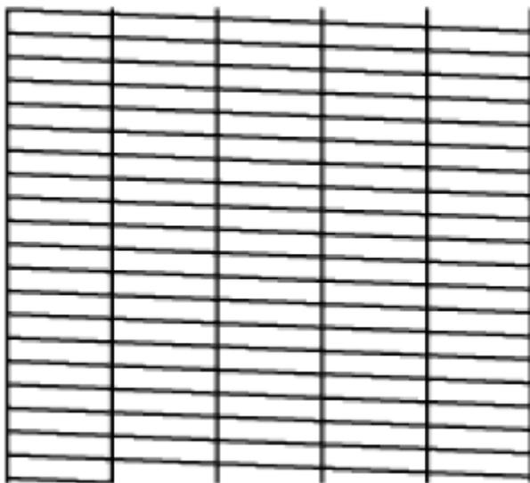
**When a print head is missing nozzles**
