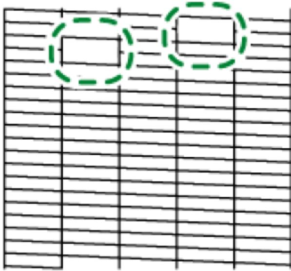
If the print head is missing nozzles, perform a Head Cleaning. See section "[Head-cleaning](#)" for more information.
