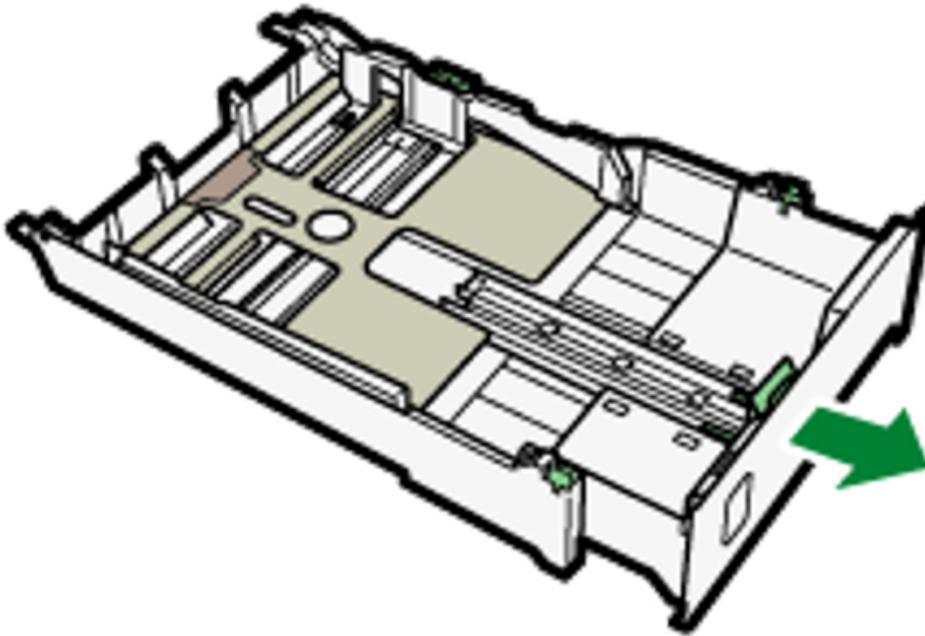
**10. Slide both tabs to the original positions, then lock the tray.**
