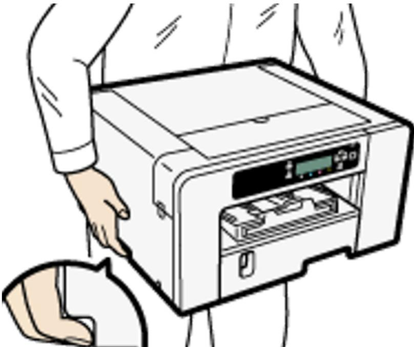
Grip the indented area at the base of the printer's sides, as shown. Lift and carry the printer slowly and carefully.
