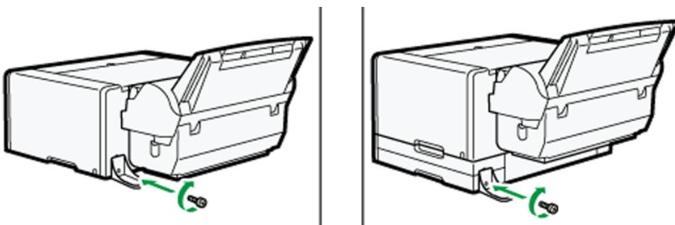
If an option tray is installed, attach the anti-topple stand to it.
