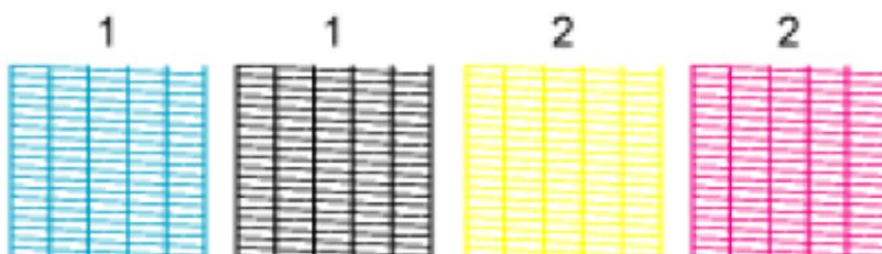
Using the printed test pattern, check for missing nozzles.
