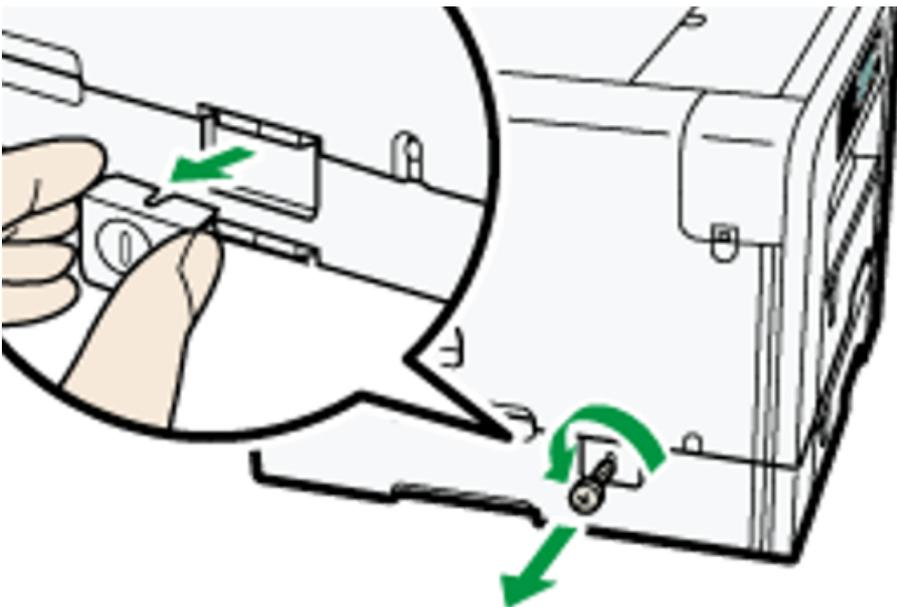
4. Temporarily move the printer to a nearby flat and stable surface to detach the option tray.
