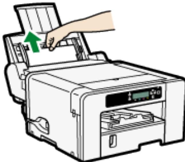
**3. Load paper / print media in the bypass tray with the side to be printed on facing up and without exceeding the sheet limit.**
