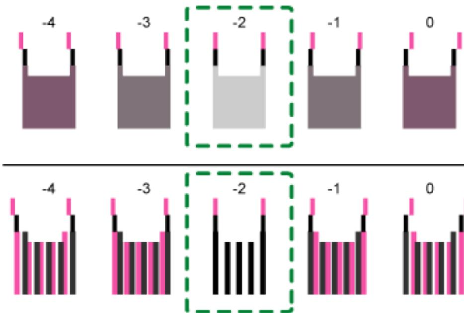
Combined two-color lines form squares, and depending on line overlapping, (white) spaces between the lines are painted and look darker. Sometimes the colors of the lines are identical.
