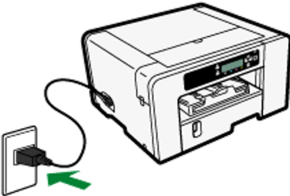
Make sure the power cord is not trapped under the printer.
