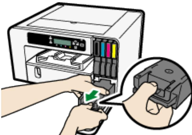
Press on the area marked "PUSH" to pull the unit out.
