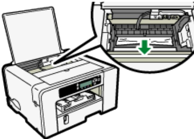
When removing the paper / print media, slowly pull it obliquely upward. Pulling it forcibly or directly upward may cause some parts to come off.
