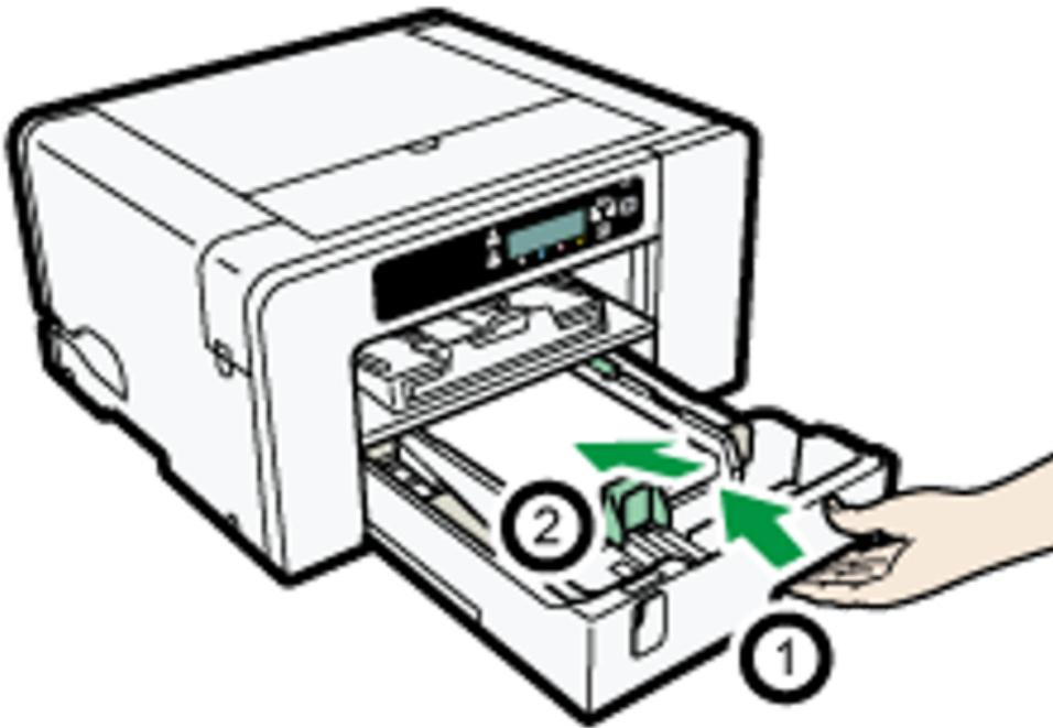
Before Tray 1 is pushed in, make sure the output ramp is closed.
