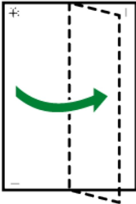
**7. The optimal adjustment value is the difference between the single vertical line and the cross's vertical line that you can see when the folded paper is held up to light. When the difference is one calibration**
