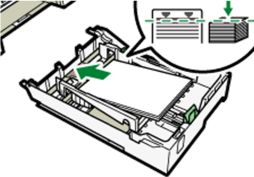
**4. Squeeze the front end paper guide, then slide it to touch the edge of the paper.**
