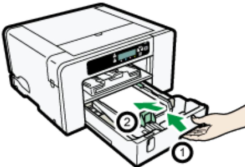
Before pushing the paper tray in, make sure the output ramp is closed.
