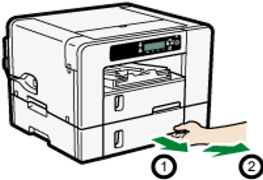
**8. Slide the tabs on both sides of the tray, then release the lock.**
