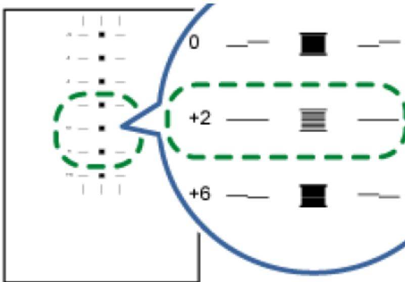
When horizontal lines beside the lightest gray square are broken, select the optimal adjustment value by referring to the lines broken in the opposite direction. When the "+2" square is the lightest gray square and the "+6" horizontal lines are broken in the opposite direction, the optimal adjustment value is between "+3" and "+5". After adjustment, check the adjustment result.
