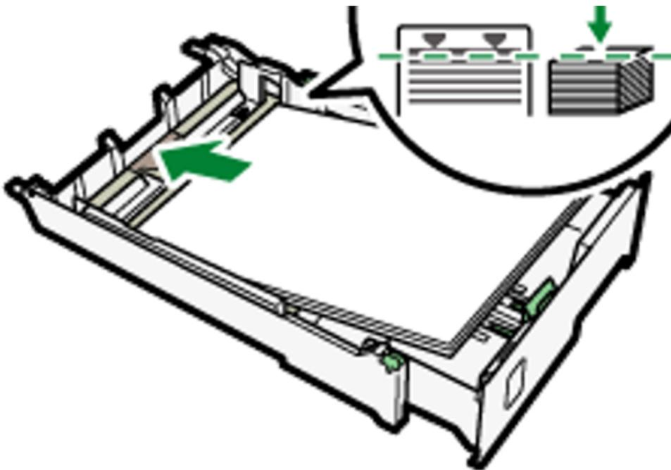
**13. Squeeze the front end paper guide, then slide it to touch the edge of the paper.**
