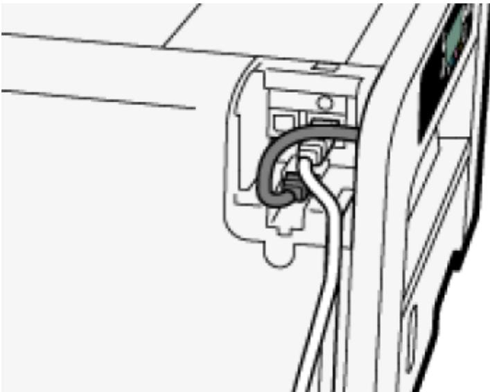
**3. Connect the other end of the cable to the printer's network, such as to a hub.**
