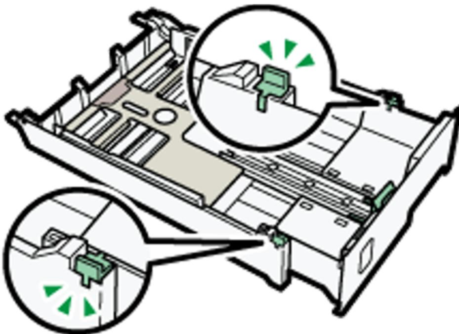
**11. Pinch the catch of the paper guide on the right side, slide the paper guides to match the size of paper /print media to load, then push the end paper guide out until there is space between them.**
