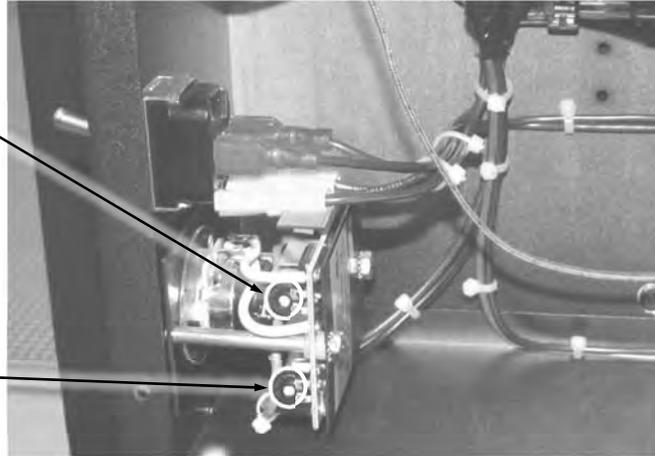
Pot near the blue wires HIGH SPEED
