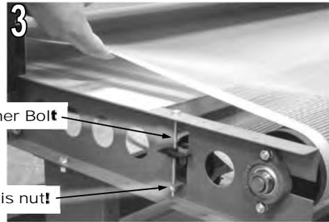
3) The belt needs to be tightened and adjusted. To tighten and adjust the belt, use the Aligner Bolts. To raise the Aligner, turn the Aligner Bolt clockwise with a 7/16" wrench. To lower it, turn it counter clockwise. Raise the Aligner until you have about 2"-2½" of slack as shown on right. Additional details on **PAGE 7**.
