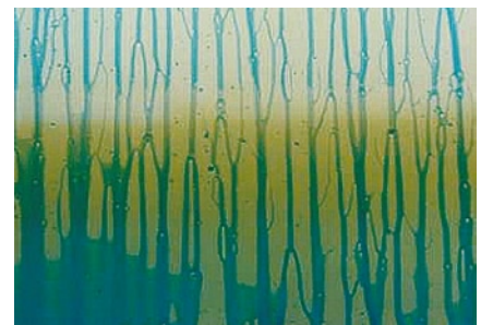
Untreated high-modulus mesh: nonuniform wetting
