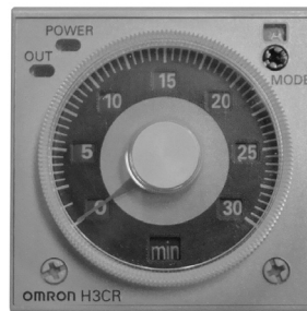
Analog Digital Timer Omron H3CR
