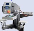
As shown on the left: the same DUPLEX MINI AUTO with its small plate (160x160) heating element installed
