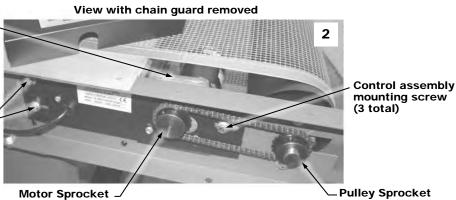
2) To adjust the drive chain you will need to loosen the three Control assembly mounting screws. The Drive plate is slotted to allow the entire assembly to slide left or right to loosen or tighten the chain. Adjust the chain so there is approximately 1/4" of vertical movement in the chain.
