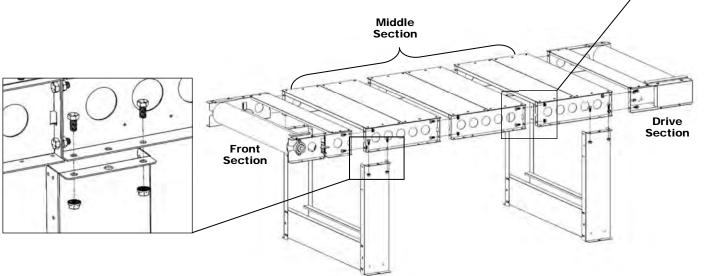
2) The belt needs to be installed as shown in the diagram. To connect your belt, align the Alligator Lace and install the pin.
