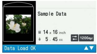
The print data loading will be completed when the print button stops blinking and remains lit, while the electric chime sounds.
