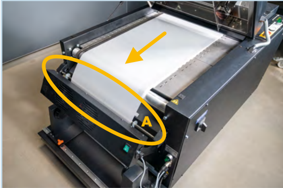
Pull the film through and lay it over the thin rod (A) on the backside of the PowDR.
