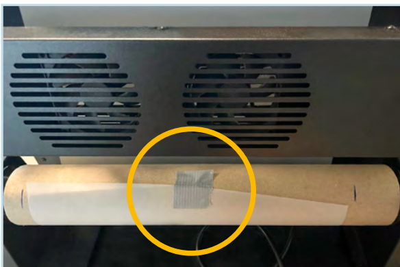
Tape the film at a point in the middle of the roll. The film can thus freely align itself a little.
