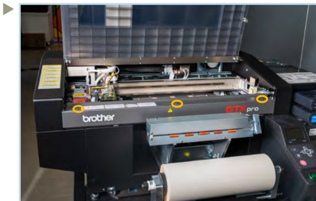
Remove the 3 screws to remove the encoder cover.
