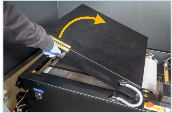
Open the big lid of the PowDR. Lift it up with the handle on the left side until it stops.
