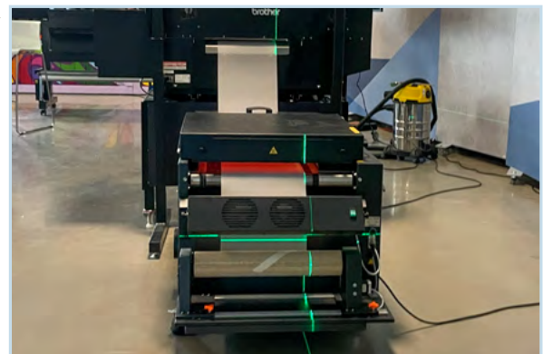
HELPFUL: Check the alignment of the film with a crossline laser.
