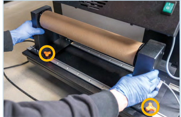
Loosen the thumbscrews and insert an empty roll that is wider than the film. Center it to the film to ensure correct winding.
